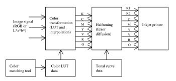
Figure 2. Signal flow of hi-fi printing
