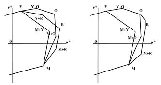
Figure 3. Schematic diagram of sub color gamuts for red region (left: original formation, right: new formation)
