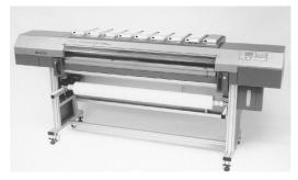
Figure 1. Textile inkjet printer Nassenger KS-1600 II
